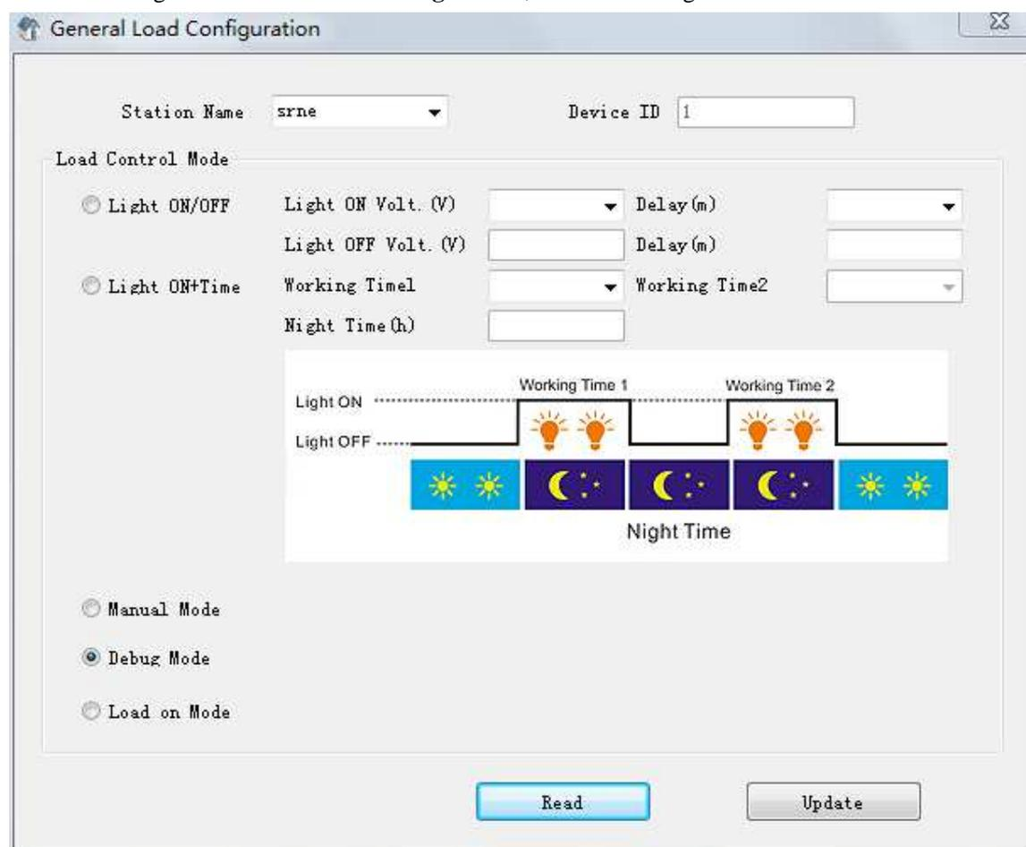
Figure 4-6-2 Dialog box **General Load Configuration**
